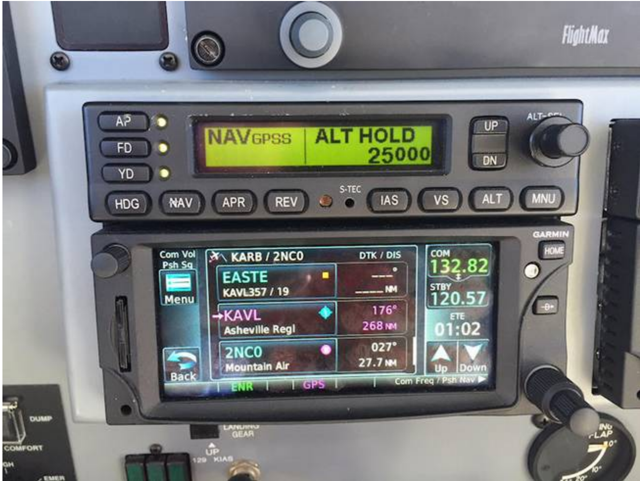
The GTN 650 makes flight plan filing and changes, frequency changes, and all other routine flight operations easy.
