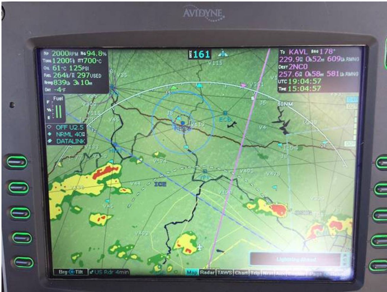
A thunderstorm at the 10:00 position was in the previous picture. Note: I deviated the aircraft to stay between the cells. Look how close I am to the cell in the Nexrad picture as opposed to the radar picture below.
